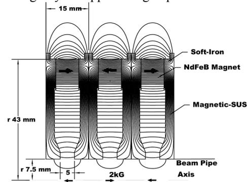
Fig. 3: Cutaway view of the PPM structure and the magnetic-field pattern.
