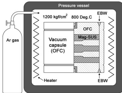
Fig. 6: HIP diffusion bonding process.
