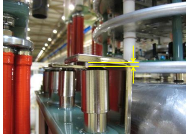
Figure 1: A disconnection point between two electrodes in an anode-modulator.
