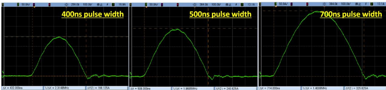
Figure 4: The CT probe signals of the output current. The vertical and horizontal axis scales are 50A/div and 100ns/div.
