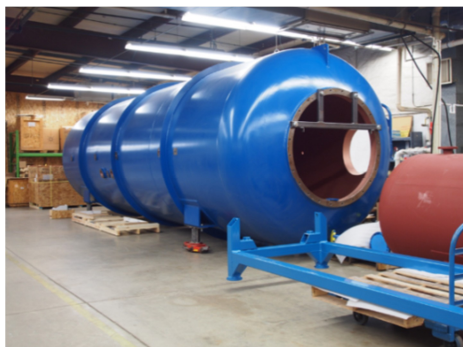
Figure 7: Photograph of the 6 MV tandem accelerator tank at the National Electrostaics Corp., USA.
