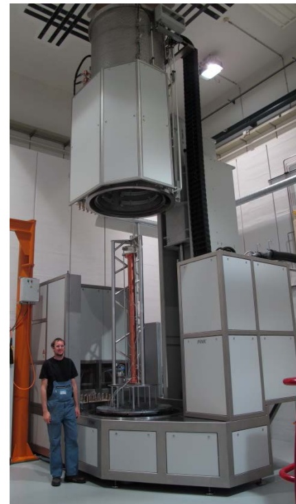
Vacuum brazing furnace installed and operative
