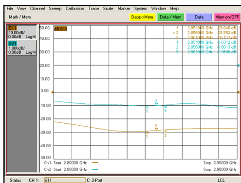
Figure 9: Measurement result of post-type combiner before shipment.
