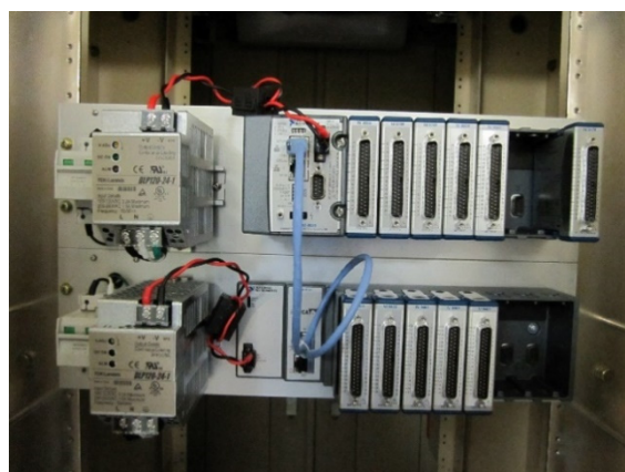
Figure 5: CompactRIO under installation. The light blue cable is used in order to interconnect the EtherCAT slave chassis (down) to the EtherCAT master controller (up).
