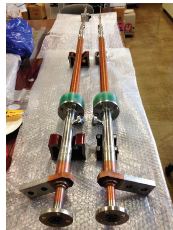
Figure 9: The current leads for the QC1E quadrupole magnets. The maximum current is 1800 A.
