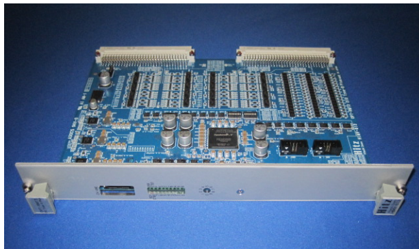
Figure 5: Photo of the newly developed OPT-RMT DIO Type-B Plus board based on the OPT-VME system.
