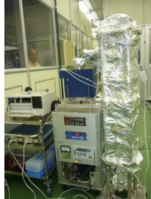
Assembly (Class 10) Baking (120°C, 48h) Hanging stand with T-map (Class 1000)
