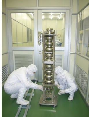
Assembly (Class 10) Baking (120°C, 48h) Hanging stand with T-map (Class 1000)
