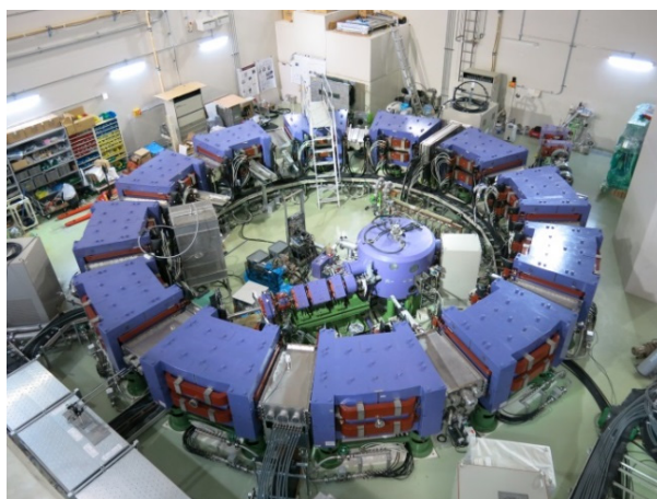
Figure 3: FFAG accelerator and beam injection line.
