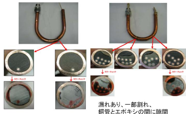
Figure 4: The penetrant inspection of the 1 signal cable(Left) and 7 signal cables in a φ12mm copper pipe.
