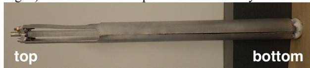
Figure 3: Thicker rod cathode.
