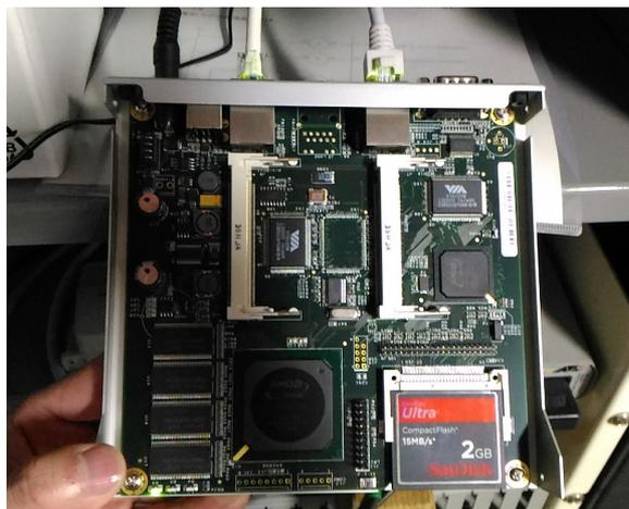
Figure 2: Photograph of ALIX single board computer. This is utilized for EPICS IOC with a gateway between Hyper ECR ion source control network and RIBF control network.
