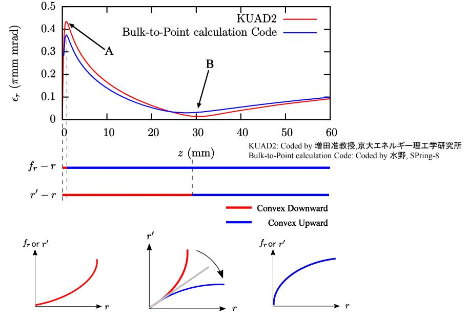
Reduction of transverse emittance in electron injectors caused by space charge effects Mizuno, A., Masuda, K., Yamamoto, M. Nuclear Instruments and Methods in Physics Research Section A: volume 774, year 2015, pp. 51 - 59
