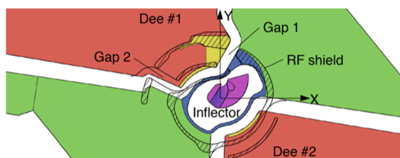
Figure 10: Existing and tested geometries of the central region. The shaded area indicates the existing geometry.
