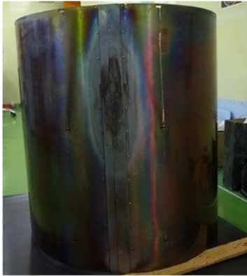
Figure 4: RF shielding cover before an improvement.
