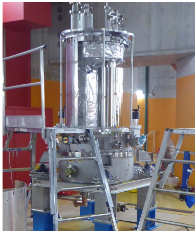
Figure 8: Assembly work of the cryomodule.
