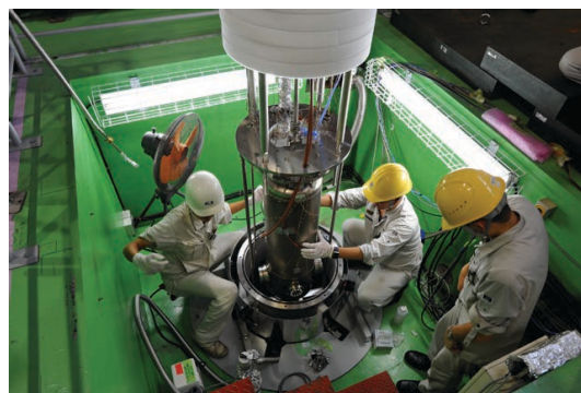
Figure 4: Installation of test assembly into the cryostat.
