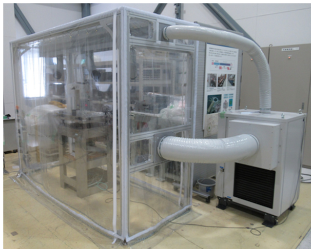
Figure 6: Temperature controlled booth for temperature coefficient measurement of permanent magnet circuit.
