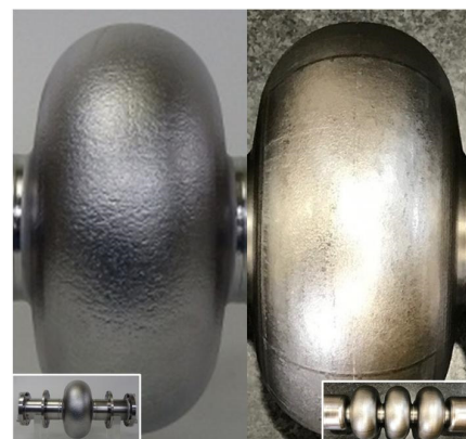
Figure 6: Comparison of cavity surface. Left) single-cell seamless cavity, Right) 3-cell seamless cavity.
