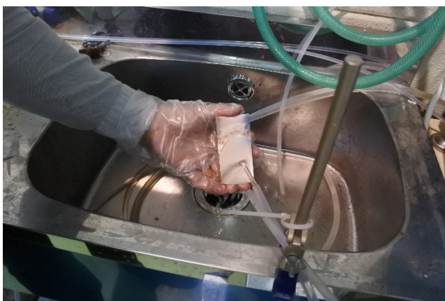
Figure 5: Ozonized water rinsing for the test piece of the copper plating.
