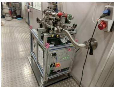
Figure 12: Picture of slow pumping system for EURO-XFEL.
