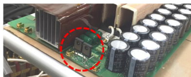
Figure 5: Printed circuit board of a MARX cell.
