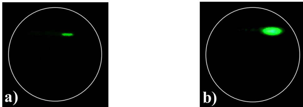
Figure 9: Photographs of the fluorescent screen during electron detection using a gas sheet. The bright spots are caused by ions that are generated by the collision of the electron beam with the gas sheet. The electron beams have a diameter of 0.35 mm for Fig.9a), and 2.0 mm for b), respectively. Write circle is added as the edge of the MCP.
