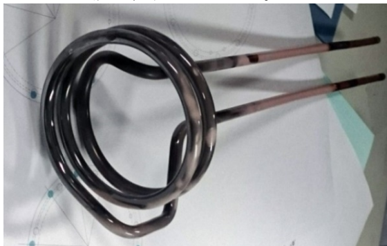
Figure 5: RF antenna after RUN#72 (1,462h) operation.
