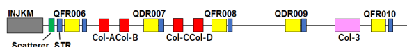
Figure 1: Collimator configuration of J-PARC MR. Boxes stand for injection kickers (gray), quadrupoles (yellow), steering magnets (blue), collimator jaws & capacitors (red/pink), and a scatterer system (green).
