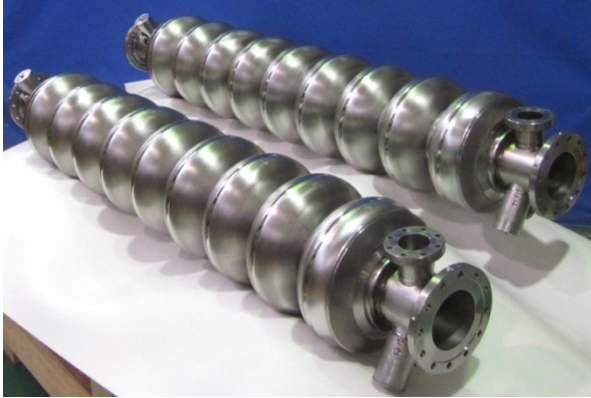
Figure 2: Picture of 9 cell TESLA cavities (TB9-TSB01, TB9-TSB02). TB9-TSB01 (front) is used for this research.
