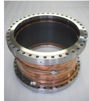
Figure 4: A KEKB type LBP damper with 4-mm thickness of ferrite, \phi 300 mm, length of 150 mm.
