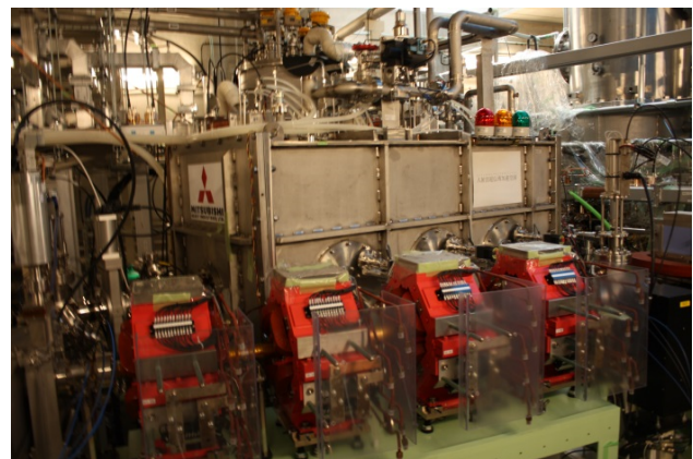
Figure 2: Injector cryomodule installed in the beam line.
