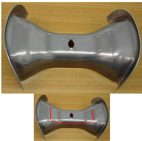
Figure 2: The 2nd Press forming test of half-spoke with 2.5 mm thick plates of aluminum. Traces of pressing were observed.
