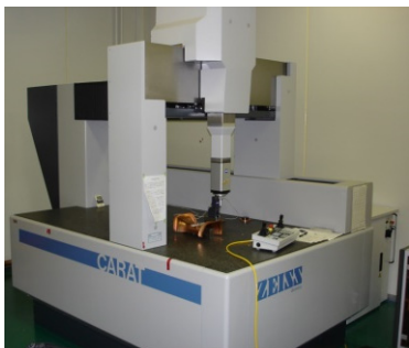
Figure 6: Precise 3D measurement device of ZEISS UPMC850 at KEK.
