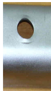
Figure 4: Traces and undulation near the bore.
