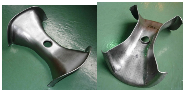
Figure 5: Press formed shape after burring with niobium sheet of 2.5 mm thick.
