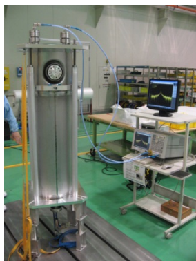
Figure 5: Frequency measurement of QWR.
