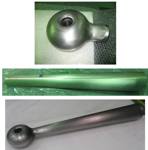
Figure 2: drift tube (top), stem (middle) and sub-assy (bottom).
