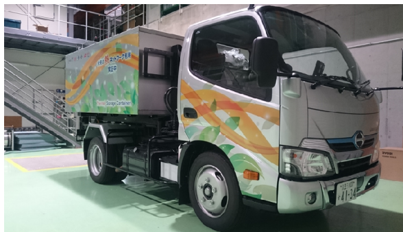
Figure 6: Adsorption thermal storage container (Hino motors truck type) [3-6].
