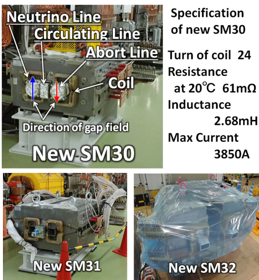
Figure 3: The new FX High-field septum magnets.
