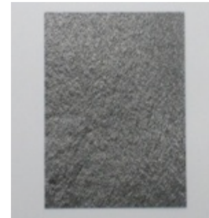
Graphite sheet 0.23 – 2.2 \text{mg}/\text{cm}^2
