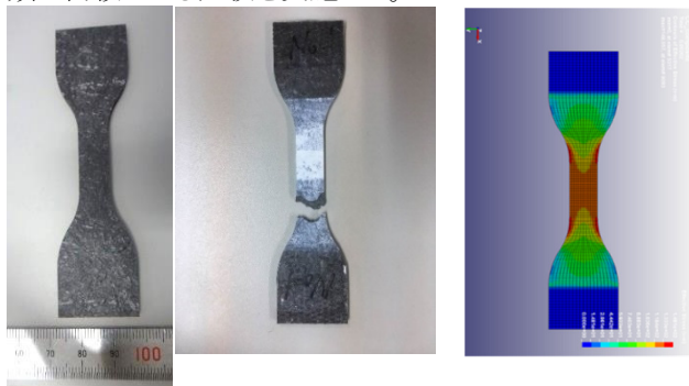
Figure 4: Tensile-test species made of C/C composite. The left and middle photographs show before and after the tensile test. The right figure shows a von-Mises stress distribution just before rupture, which is calculated by the LS-DYNA.
