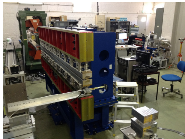
Figure 5: Photograph of U01 during the magnetic measurement.
