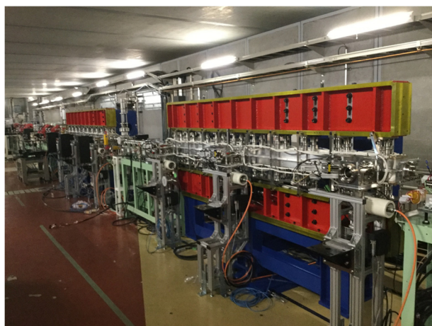
Figure 1: Photograph of the cERL-FEL undulator.
