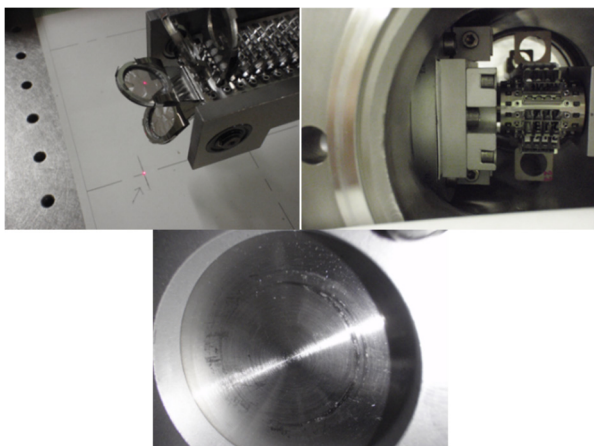
Figure 8: Photo of the foil changer mechanism. Below is a photograph of the scratch marks on the vacuum partition. Down) Rubbing marks on the vacuum partition.
