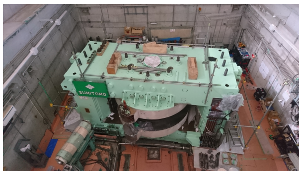
Figure 2: The AVF cyclotron being disassembled. The yokes, the poles, and the main coils are continued to be used after the upgrade.
