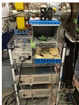
Figure 5: Photograph of RFKO system.
