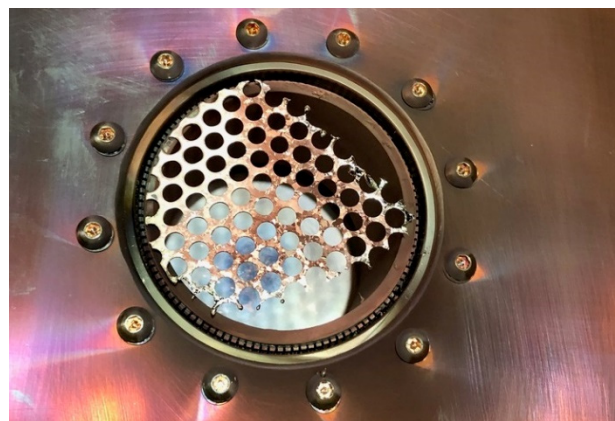
Figure 3: Damaged RF shield.
