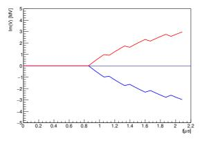
Figure 10: The imaginary part of RF term (red) and Beam term (blue) with the input RF phase modulation and the amplitude moduelation on the gap. The RF term and beam term repeated the cycle of grwoth and decay depending on the pulse structure. Their amplitude are same with different sign.
