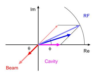
Figure 4: Phase diagram of RF term (blue) and Beam term (red) with phase  $\theta$  after the phase modulation of the input RF with  $\phi$ . The solid and hatched arrows show the instantinous and the asymptotic values.
