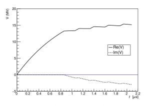
Figure 7: Cavity voltage variation with the input RF phase modulation, but no treatment on the gap. The cavity voltage is increased in the gap.
