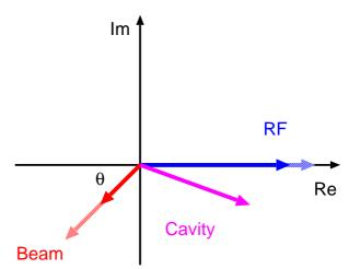
Figure 3: Phase diagram of RF term (blue) and Beam term (red) with phase  $\theta$ . The solid and hatched arrows show the instantinous and the asymptotic values.
