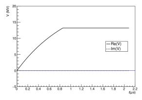
Figure 8: Cavity voltage variation with the input RF phase modulation including the amplitude modulation on the gap. The cavity voltage is maintained as a constant. The solid and dashed lines are the real and imaginary components. The imaginary components is not appeared at all.
