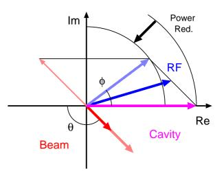
Figure 5: Phase diagram of RF term (blue) and Beam term (red) with phase  $\theta$  after the phase modulation of the input RF with  $\phi$ . The solid and hatched arrows show the instantinous and the asymptotic values. If  $\theta > \pi/2$ , the input power should be also modulated (less power).
