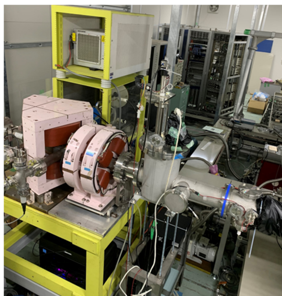
Figure 1: Schematic view of proton generator using NANOGAN. Only 3\text{He}^{2+} can be introduced into the reaction chamber at the end of this system with using dipole magnet and quadrupole magnets.
