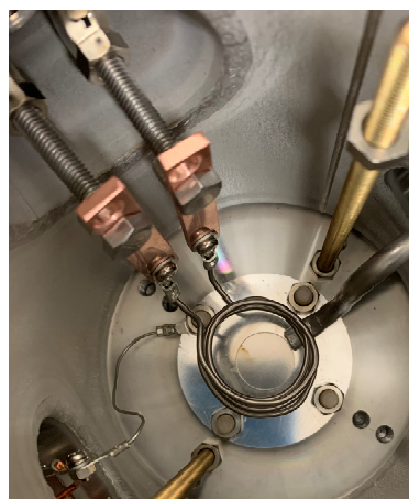
Figure 7: Schematic view of evaporation system with 2 mm Ti wire.
