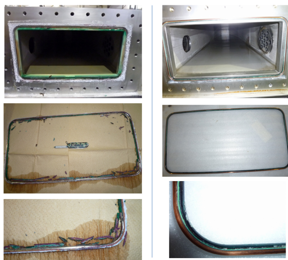
Figure 3: Comparison of damages dependent on the water quality around metal seal checked after the KEKB operation.
