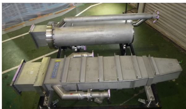
Figure 1: High-power water-loads (Upper: Cylindrical-waveguide type, bottom: rectangular waveguide type).
