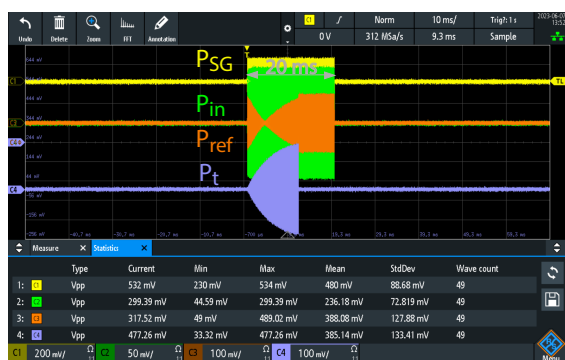
Figure 13: RF signals observed during pulsed rf power conditioning.
