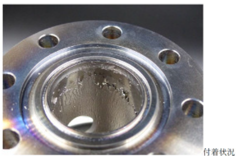
Figure 5: Photograph of the position near the beam pipe tube of the Nb coupon cavity after DC magnetron sputtering.
