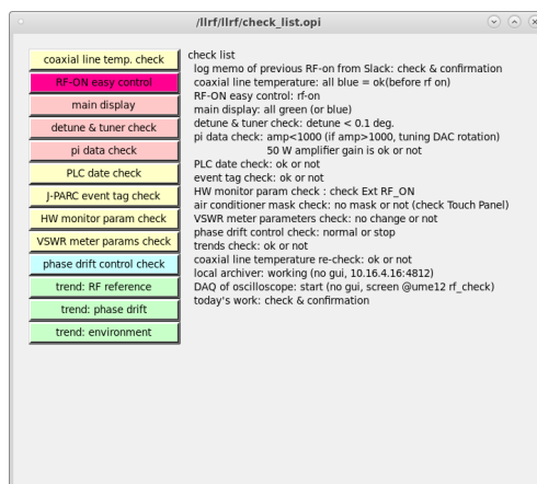
Figure 2: GUI for the RF startup with the check list and the control launcher.
