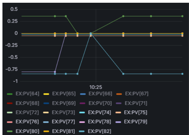
Figure 3: Visualized array data with timeseries format on Time series panel. Only the last 9 elements in the array are shown in this plot.
