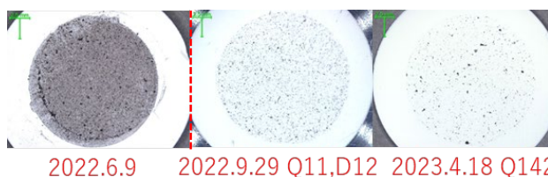
Figure 4: Filter images after cooling water filtration.
