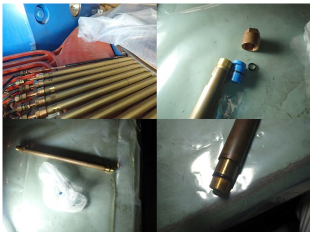
Figure 6: Feedthrough pipes of trim coils and hardening of an O-ring at C8-OUT.
