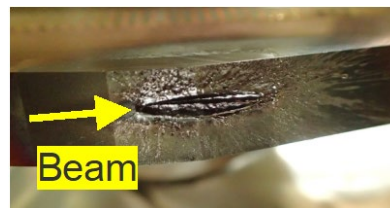
Figure 2: Collimator head damaged by SBL.
